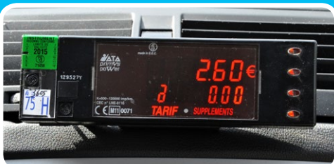
a time-distance meter indicating the rate and journey fare
